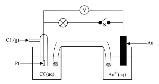
With switch **S** OPEN, the initial reading on the voltmeter is 0,14 V.
