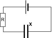
Capacitor **X** is now replaced with a similar capacitor, **Y**, with the same dimensions but with paper between its plates. When fully charged, the charge stored on the plates of capacitor **Y** is ...
