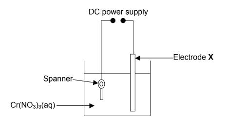
A constant current passes through the  $Cr(NO_3)_3(aq)$  solution and its concentration remains constant during the process. In the process, a total of 0,03 moles of electrons is transferred in the electrolytic cell.
