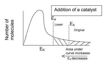
A catalyst provides an alternative pathway for the reaction which has a lower  $E_a$ . With the catalyst more molecules have  $E_K$  greater than or equal to  $E_a$  (Shaded area under the curve is larger). There are more effective collisions per unit time. Therefore the addition of a catalyst increases reaction rate.
