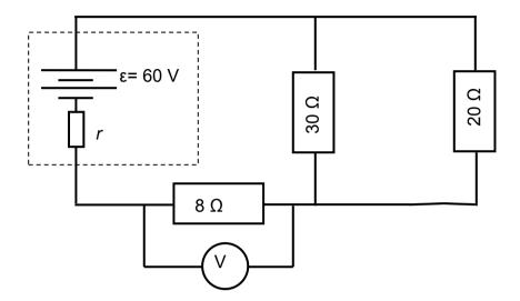
A voltmeter connected across the 8  $\Omega$  resistor reads 21,84 V.
