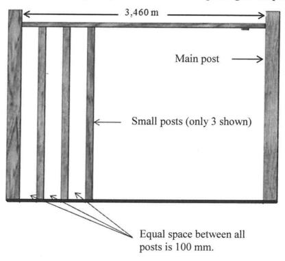
**NOTE:** A small post has a width of 40 mm. The spaces between the posts in the panel is 100 mm.
