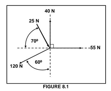
**HINT:** To assist you, draw and complete the force diagram shown in FIGURE 8.1. Show ALL the horizontal (HC) and vertical components (VC) before you do the calculations.
