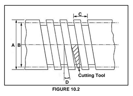
10.3 Explain how the sides of cutting tools must be ground in order to cut a square thread.
