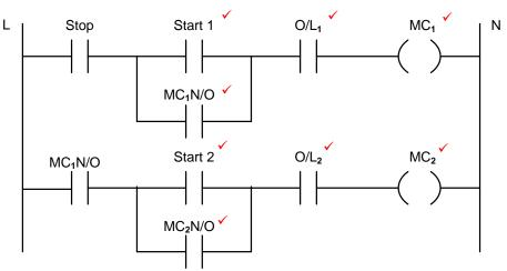
**NOTE:** Alternatively, the candidate could use closed symbols in the place of the open stop symbol and both overload symbols. Stop and overload symbols must be in the same normal state. (8)
