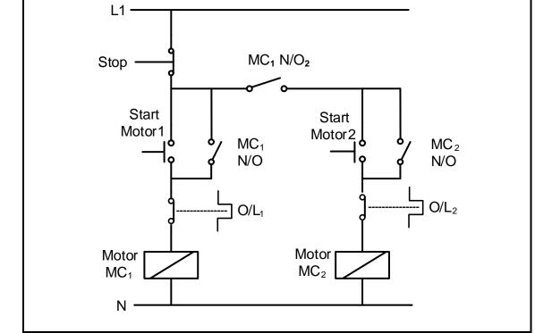
FIGURE 7.6: MANUAL SEQUENCE STARTER WITHOUT A TIMER
