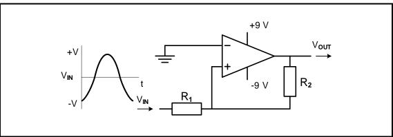
FIGURE 5.4: NON-INVERTING SCHMITT TRIGGER
