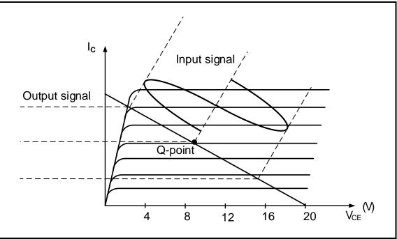
**FIGURE 6.2: CLASSES OF AMPLIFICATION**
