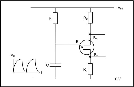
FIGURE 4.5: THE UJT AS A SAW-TOOTH GENERATOR
