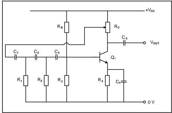
FIGURE 6.9: RC PHASE-SHIFT OSCILLATOR
