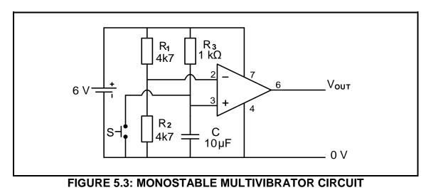
5.3.1 Determine the voltage at pin 2 (inverting input) of the op amp.
