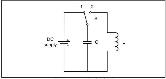
FIGURE 6.6: TANK CIRCUIT
