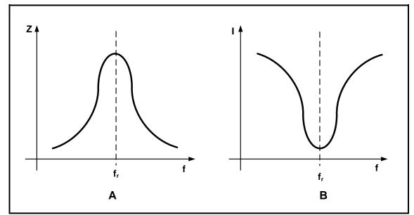
FIGURE 3.5: IMPEDANCE AND CURRENT RESPONSE CURVES
