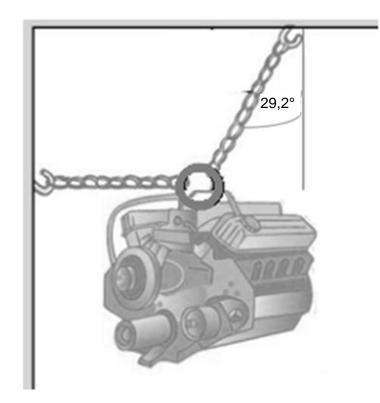
The forces acting on the engine are represented by the following free body diagram:
