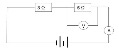
Calculate the potential difference across the 5  $\Omega$  resistor. (5) [10]
