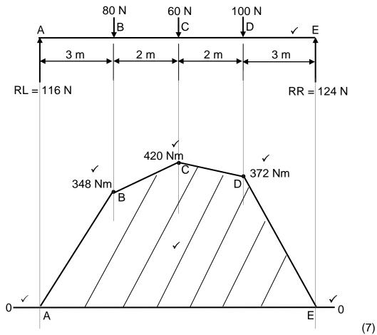
**NOTE:** Draw the bending moment diagram to scale for marking purposes.
