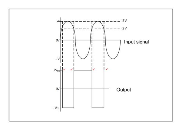
7.4 Audio application where the signal must be inverted ✓
